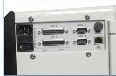
**New External Connectivity 12 inputs/ 12 outputs I/O Options**
